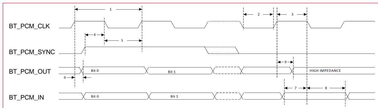
**Table 16: Long Frame Sync Signal Parameters - Slave Mode**
