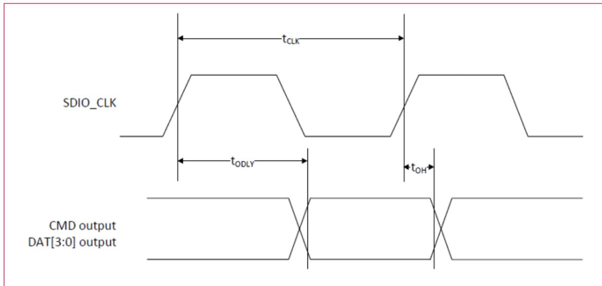
Table 22: DIO Bus Output Timing Parameters - SDR Modes up to 100 MHz
