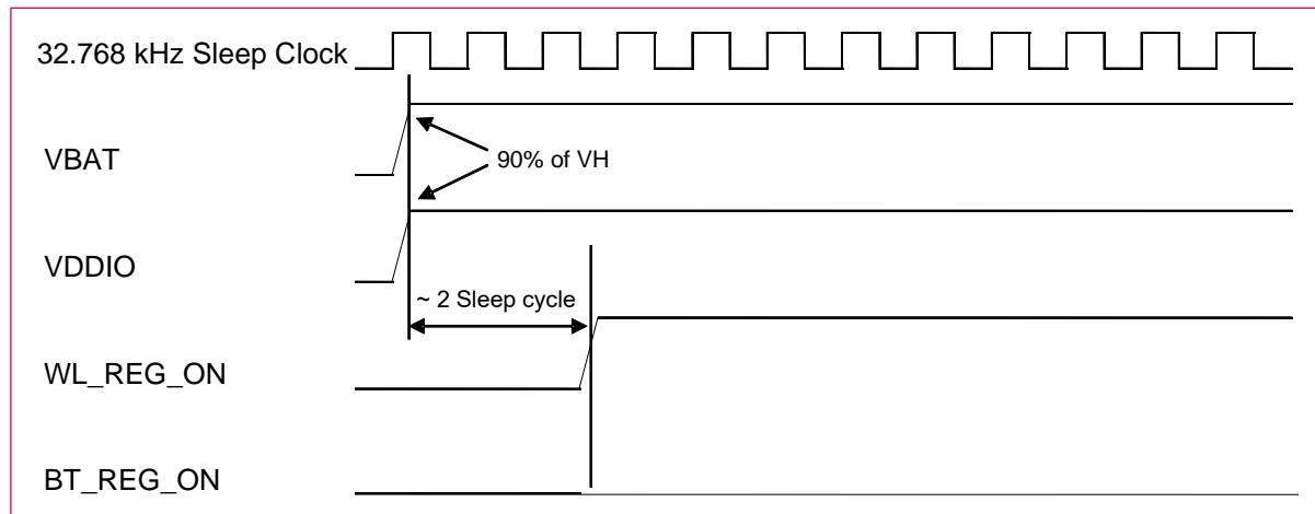
**Figure 9** shows the power-on sequence for WLAN OFF and BT ON.
