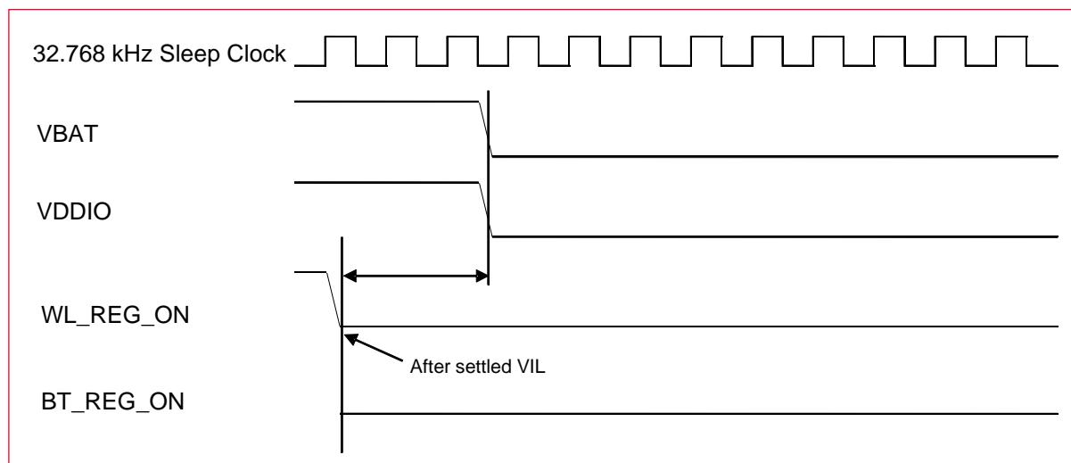
**Figure 13**Figure 12 shows the power-off sequence for WLAN OFF and BT ON.
