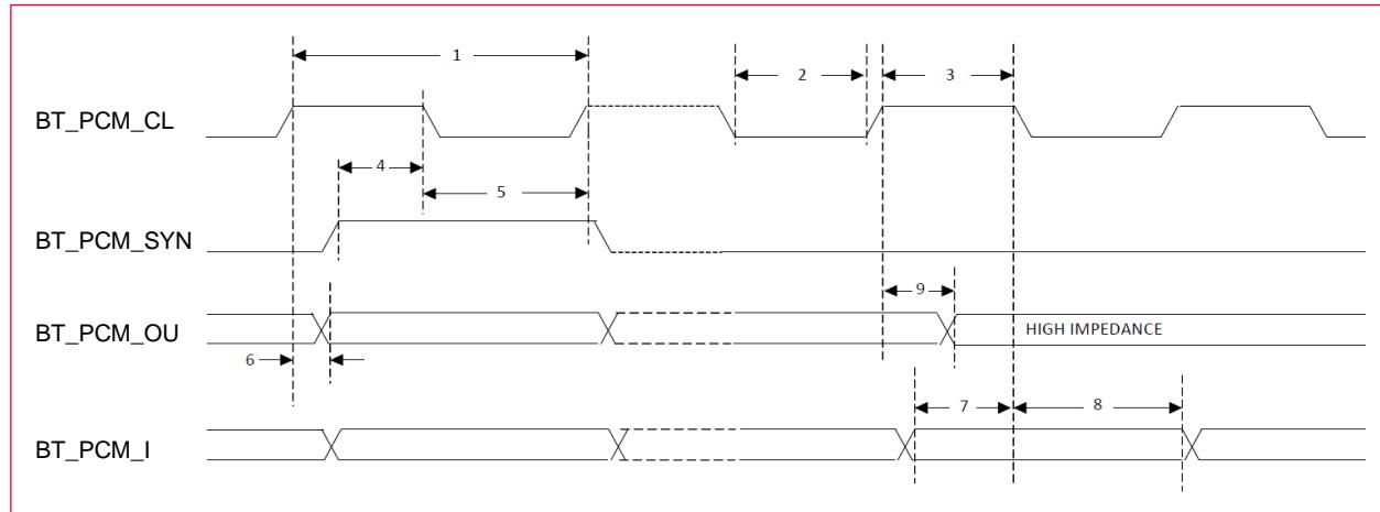
**Table 14: Short Frame Sync Signal Parameters - Slave Mode**
