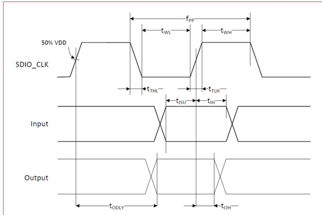
**Table 19: SDIO Bus Timing Parameters - High-Speed Mode**
