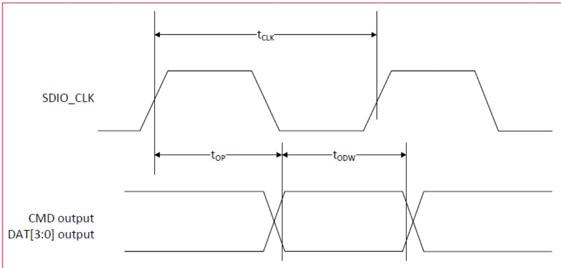
**Table 23: SDIO Bus Output Timing Parameters - SDR Modes 100 MHz to 208 MHz**
