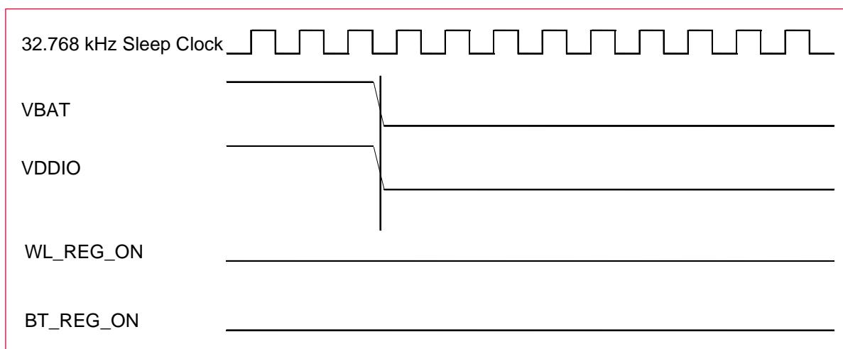
**Figure 12** shows the power-off sequence for WLAN ON and BT OFF.
