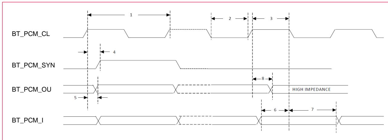
**Table 13: Short Frame Sync Signal Parameters - Master Mode**
