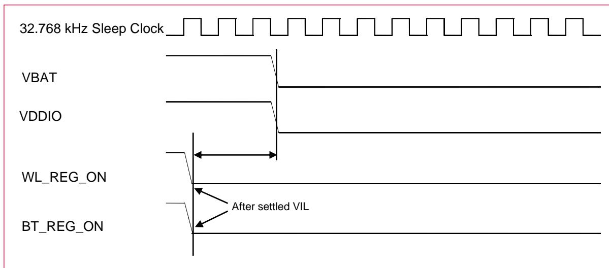
**Figure 11** shows the power-off sequence for WLAN OFF and BT OFF.
