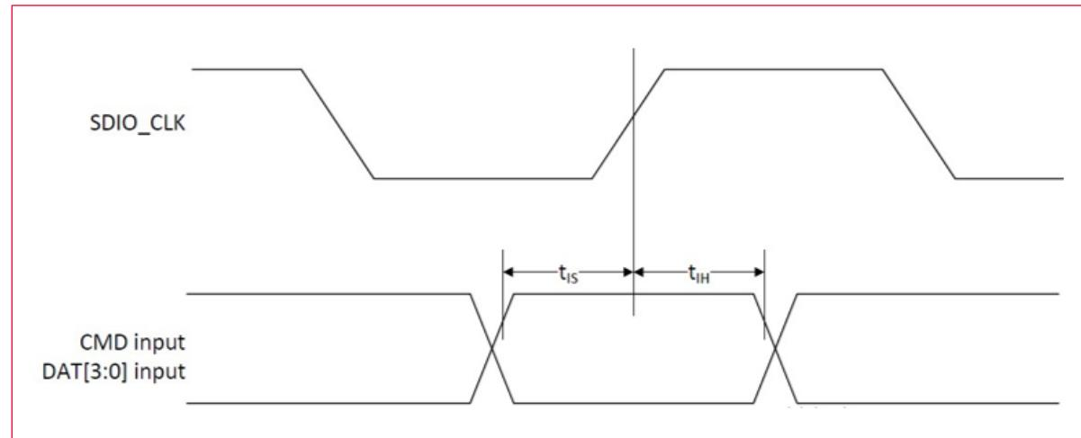
**Table 21: SDIO Bus Input Timing Parameters - SDR Modes**
