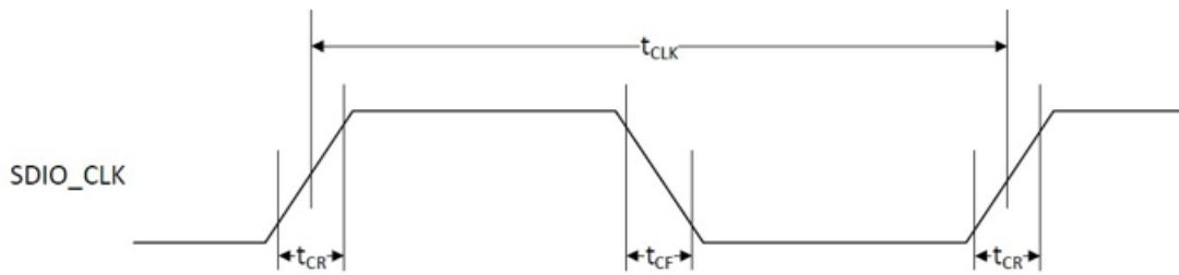
**Table 20: SDIO Bus Clock Timing Parameters - SDR Modes**
