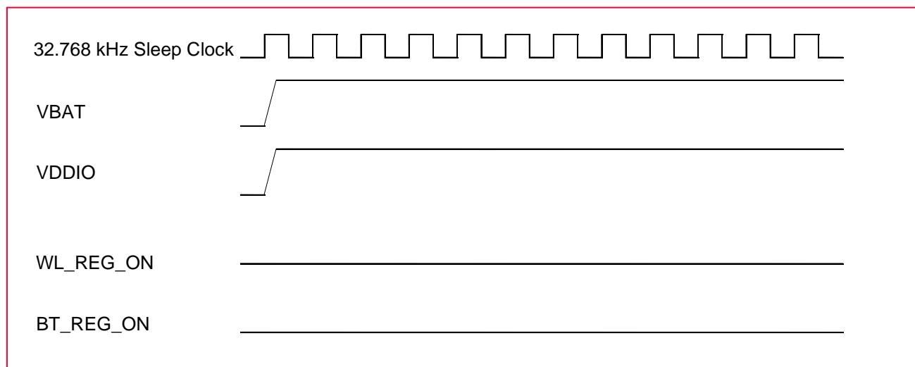
**Figure 8** shows the power-on sequence for WLAN ON and BT OFF.
