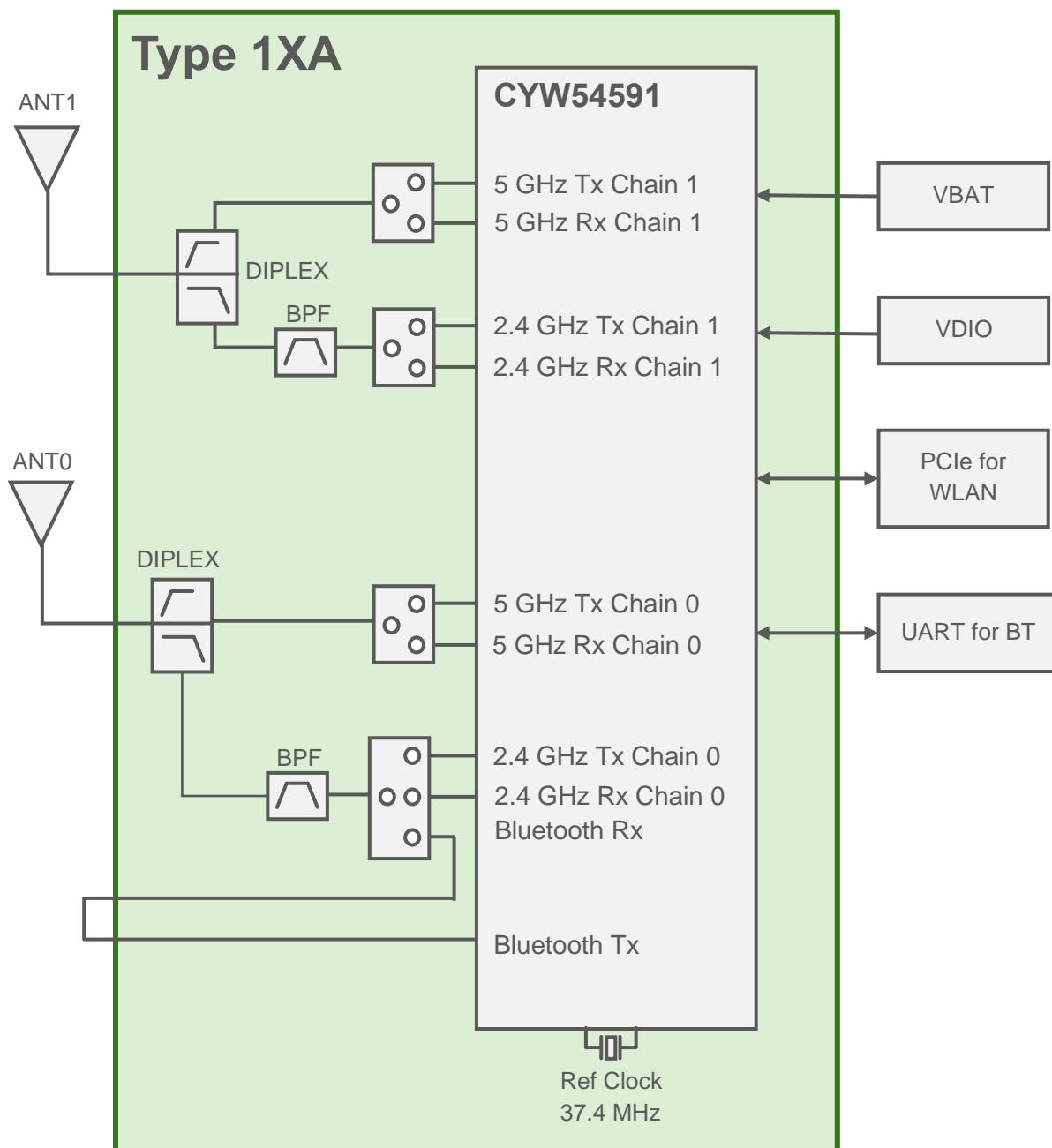
Figure 2: Type1XA Block Diagram for Three Antenna Configuration
