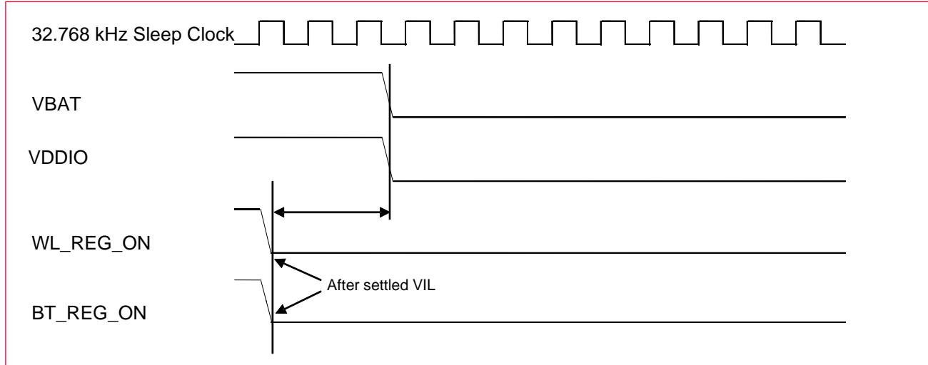
**Figure 11** shows the power-off sequence for WLAN OFF and BT OFF.
