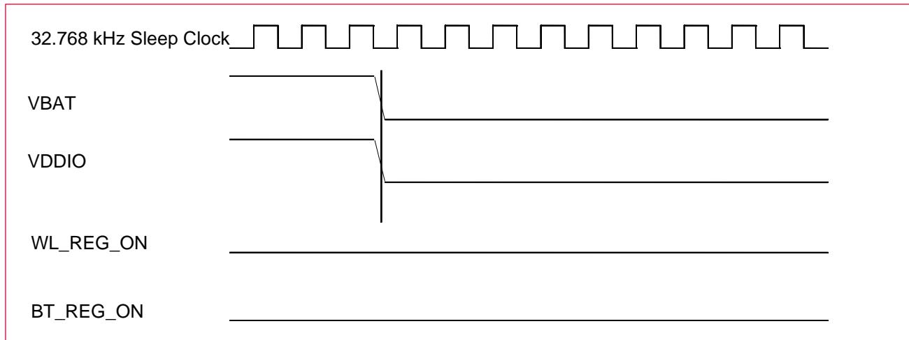
**Figure 12** shows the power-off sequence for WLAN ON and BT OFF.
