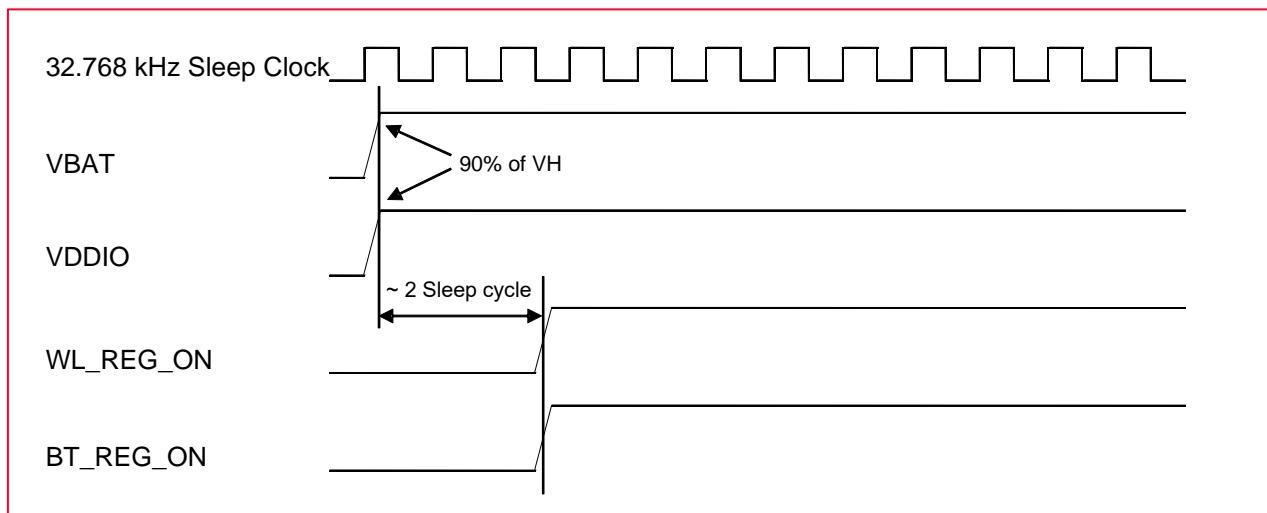
**Figure 7** shows the power-on sequence for WLAN OFF and BT OFF.
