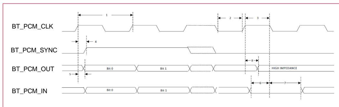
**Table 15: Long Frame Sync Signal Parameters - Master Mode**
