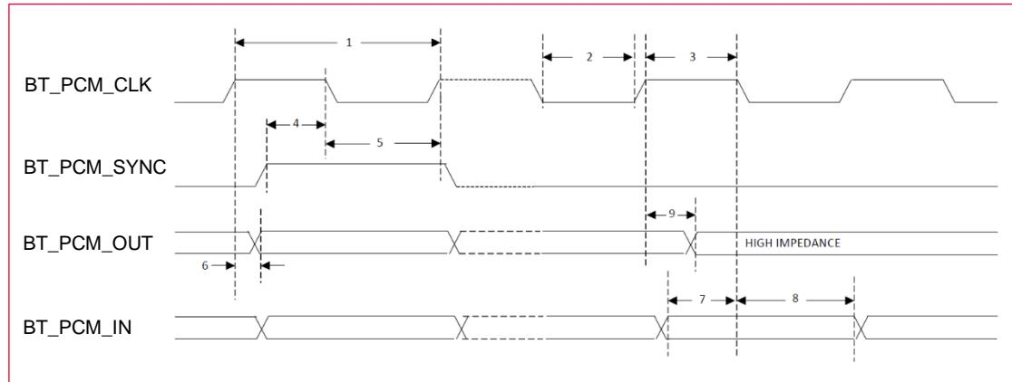
**Table 14: Short Frame Sync Signal Parameters - Slave Mode**
