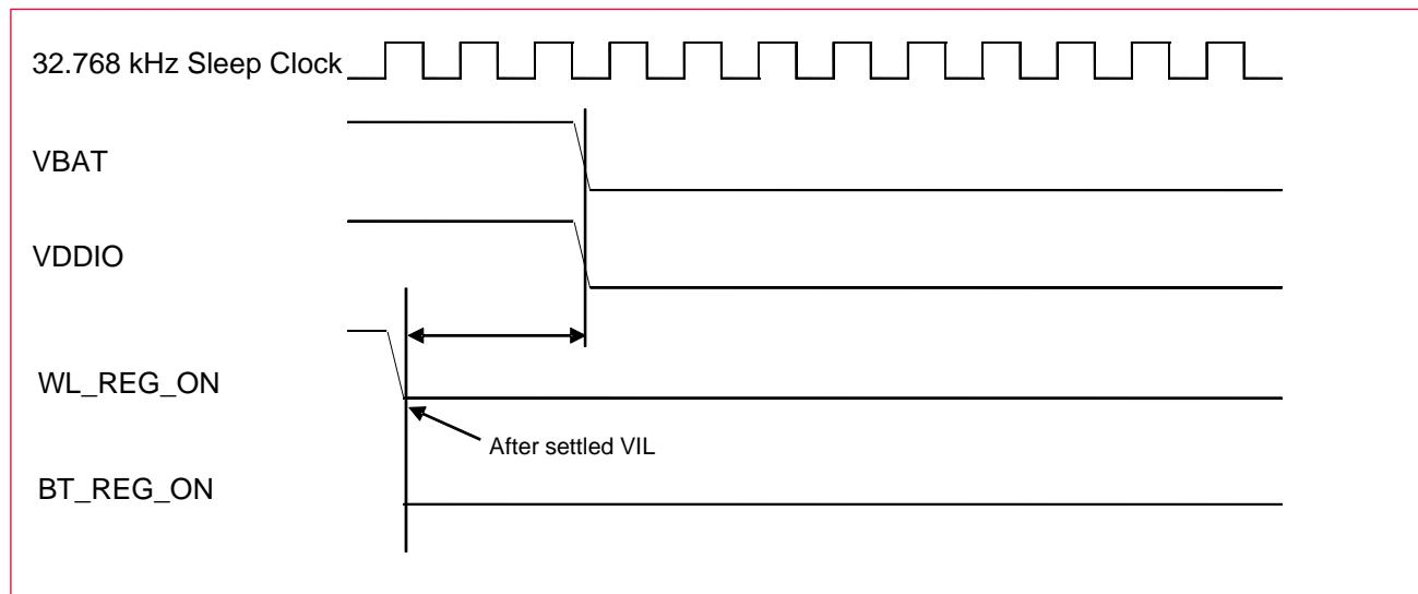
**Figure 13** shows the power-off sequence for WLAN OFF and BT ON.
