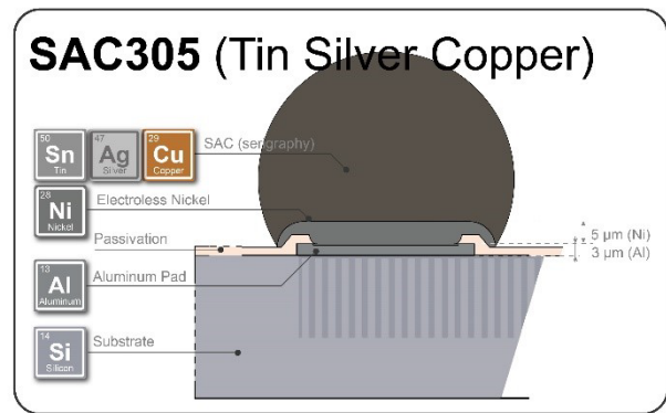
Figure 7 – Top electrode description of SAC305 pre-bumped version
