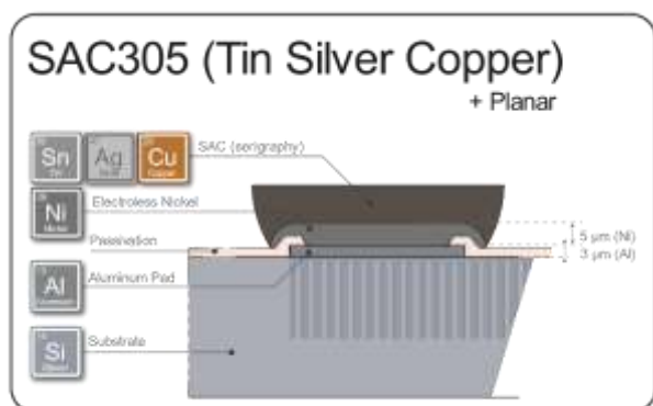
Figure 6 – Top electrode description of SAC305 pre-bumped version
