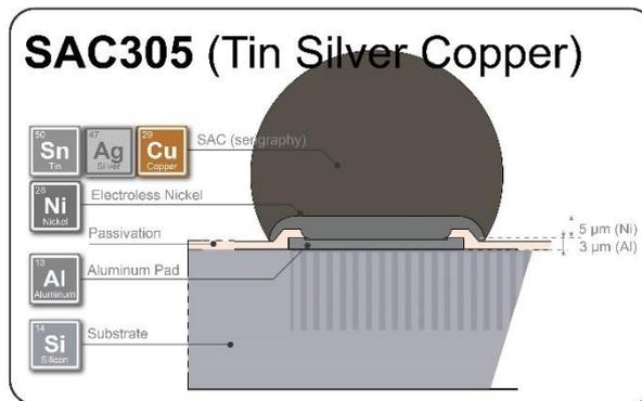
Figure 7 – Top electrode description of SAC305 pre-bumped version
