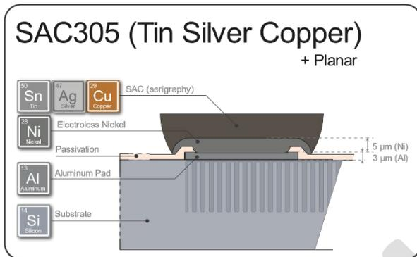
Figure 6 – Top electrode description of SAC305 pre-bumped version
