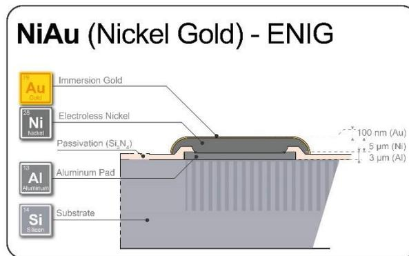
Figure 7 – Top electrode description of ENIG finishing version
