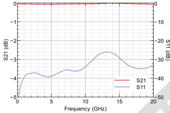
Figure 2 - 47nF ULSC Measured results (module of S-parameters)
