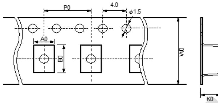
Figure 13 – Tape drawing (not to scale)
