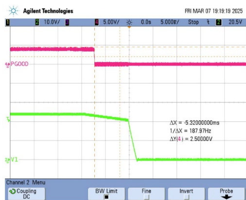
PWR_OK vs V1 at turn on 100% load, 230Vac
