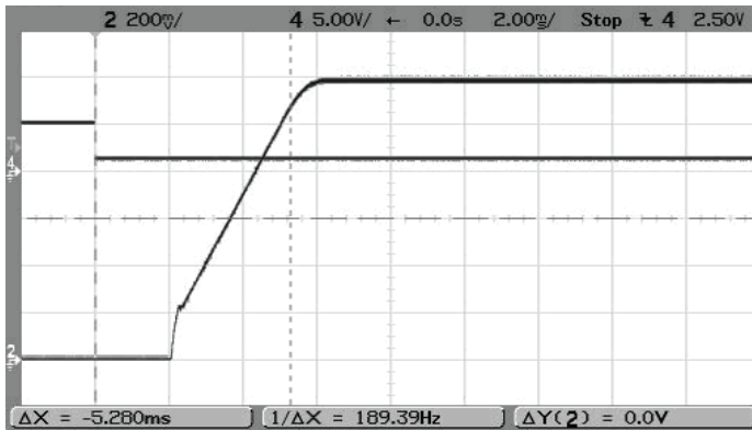
Step Load Transient Response (Vin = 5V, Vout = 1.2V, Clload = 0, Iout = 1.5 to 3A) Trace 2 = Vout, 100 mV/div. Trace 4 = Iout, 2.5A/div.
