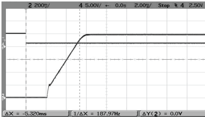
Step Load Transient Response (Vin = 5V, Vout = 1.0V, Cload = 0, Iout = 1.5 to 3A) Trace 2 = Vout, 100 mV/div. Trace 4 = Iout, 2.5A/div.
