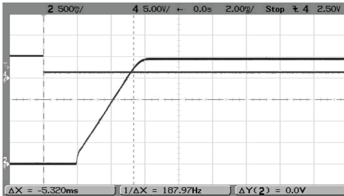
Step Load Transient Response (Vin = 5V, Vout = 2.5V, Clload = 0, Iout = 1.5 to 3A) Trace 2 = Vout, 100 mV/div. Trace 4 = Iout, 2.5A/div.
