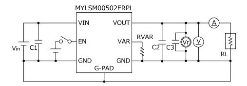
Vin: DC Power Supply RL: Electronic Load Device
