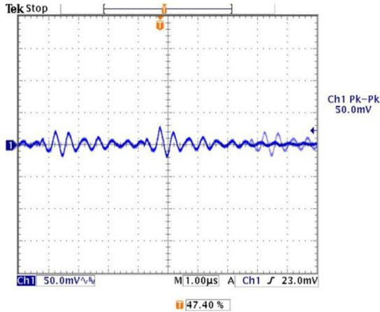
Output Ripple and Noise (Vin=24V, Vout=nom., Iout=2A, Cload=1μF ceramic || 10μF tantalum, Ta=+25°C., ScopeBW=20MHz)
