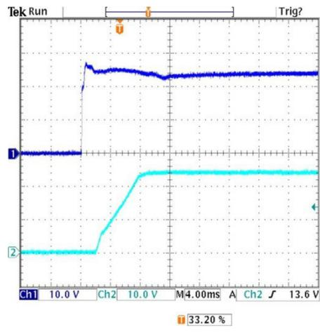
Pre-biased output voltage added connecting an external  $680\mu F$  to the output ( $V_{in}=24V$ ,  $I_{out}=0A$ ,  $+25^\circ C$ )
