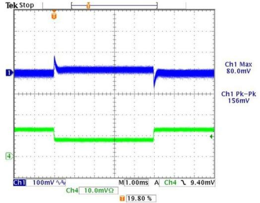
Power On Startup Delay ( $V_{in}=0$  to  $24V$ ,  $V_{out}=nom.$ ,  $I_{out}=no$  load,  $C_{load}=0\mu F$ ,  $T_a=+25^\circ C$ , ScopeBW=20MHz) Trace 1= $V_{in}$ , Trace 2= $V_{out}$
