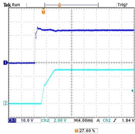
Pre-biased output voltage added connecting an external 5000µF to the output ( $V_{in}=24V$ ,  $I_{out}=0A$ ,  $+25^\circ C$ )
