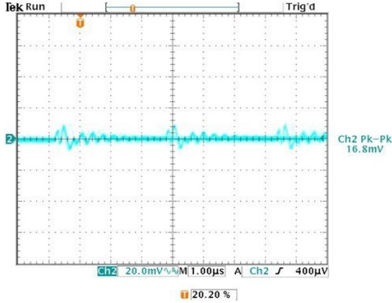
Output Ripple and Noise (Vin=24V, Vout=nom., Iout=4.5A, Cload=1μF ceramic II 10μF tantalum, Ta=+25°C., ScopeBW=20MHz)
