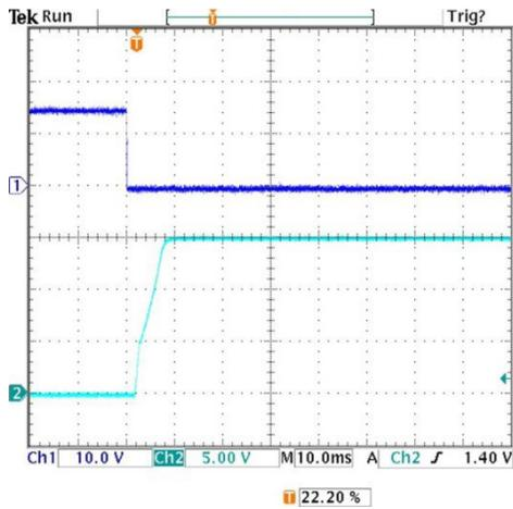
On/Off Enable Delay (Negative logic, Vin=24V, Vout=nom., Iout=3.3A, Cload=0μF, Ta=+25°C., ScopeBW=20MHz) Trace 1=Enable, Trace 2=Vout
