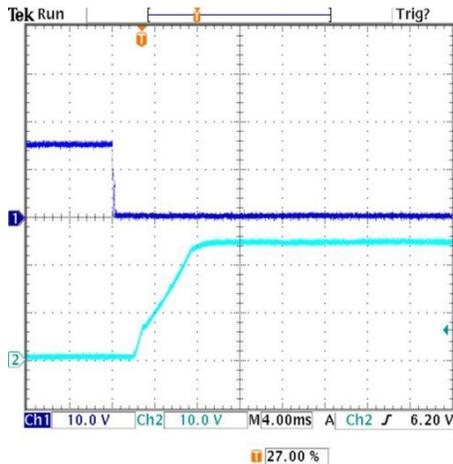
On/Off Enable Delay (Negative logic, Vin=24V, Vout=nom., Iout=2A, Cload=0 μF, Ta=+25°C., ScopeBW=20MHz) Trace 1=Enable, Trace 2=Vout
