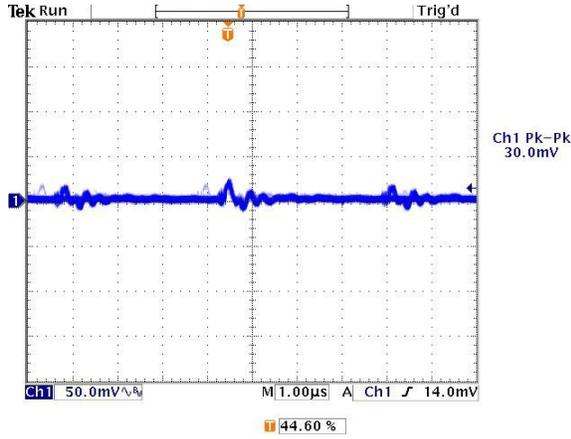
Output Ripple and Noise (Vin=24V, Vout=nom., Iout=3.3A, Cload=1μF ceramic II 10μF tantalum, Ta=+25°C., ScopeBW=20MHz)
