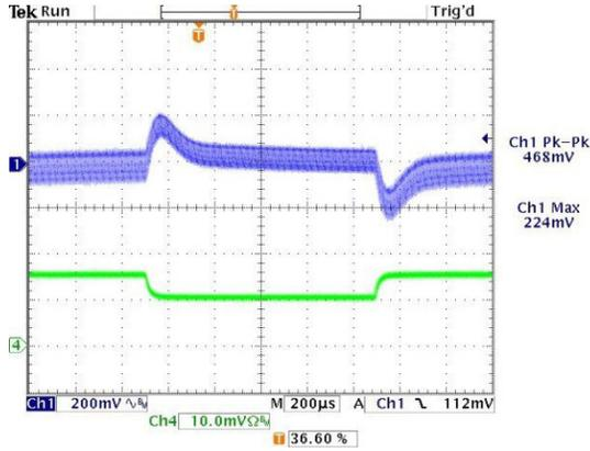
Step Load Transient Response ( $V_{in}=24V$ ,  $V_{out}=nom.$ ,  $I_{out}=50-75-50\%$  of full load,  $C_{load}=2000\mu F$ ,  $T_a=+25^\circ C$ , ScopeBW=20MHz)
