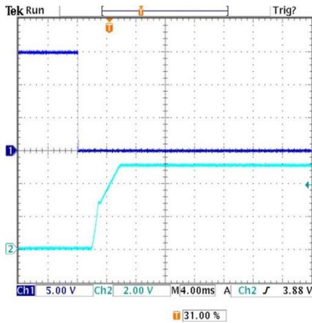
On/Off Enable Delay (Negative logic, Vin=24V, Vout=nom., Iout=10A, Cload=0 μF, Ta=+25°C., ScopeBW=20MHz) Trace 1=Enable, Trace 2=Vout
