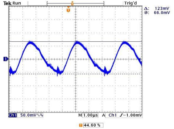
On/Off Enable Delay (Negative logic, Vin=24V, Vout=nom., Iout=no load, Cload=0μF, Ta=+25°C., ScopeBW=20MHz) Trace 1=Enable, Trace 2=Vout
