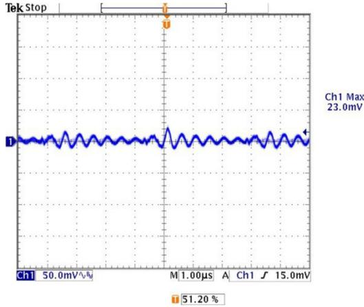
Output Ripple and Noise (Vin=24V, Vout=nom., Iout=15A, Cload=1μF ceramic || 10μF tantalum, Ta=+25°C., ScopeBW=20MHz)
