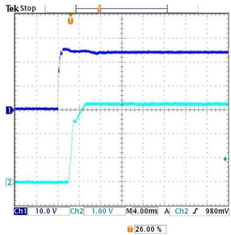
Pre-biased output voltage added connecting an external 10000µF to the output ( $V_{in}=24V$ ,  $I_{out}=0A$ ,  $+25^\circ C$ )
