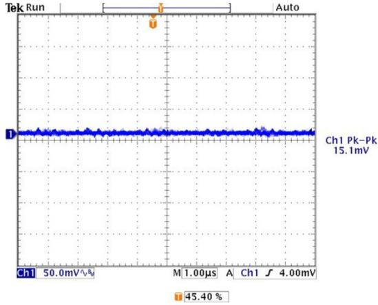
Output Ripple and Noise (Vin=24V, Vout=nom., Iout=10A, Cload=1μF ceramic || 10μF tantalum, Ta=+25°C., ScopeBW=20MHz)
