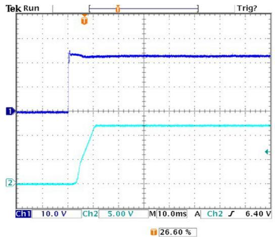
Pre-biased output voltage added connecting an external 2000uF to the output ( $V_{in}=24V$ ,  $I_{out}=0A$ ,  $+25^\circ C$ )
