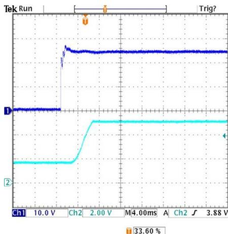
Pre-biased output voltage added connecting an external supply through a diode ( $V_{in}=24V$ ,  $I_{out}=0A$ ,  $+25^\circ C$ )
