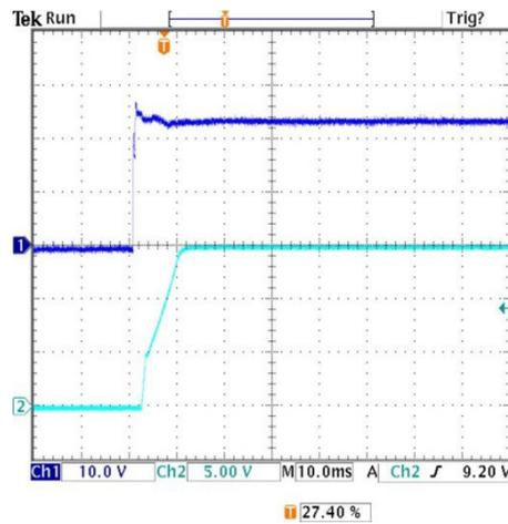
Pre-biased output voltage added connecting an external  $2000\mu F$  to the output ( $V_{in}=24V$ ,  $I_{out}=0A$ ,  $+25^\circ C$ )
