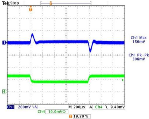
Step Load Transient Response ( $V_{in}=24V$ ,  $V_{out}=nom.$ ,  $I_{out}=50-75-50\%$  of full load,  $C_{load}=5000\mu F$ ,  $T_a=+25^\circ C$ , ScopeBW=20MHz)
