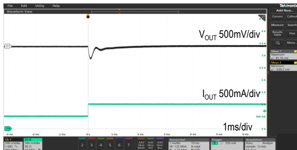
Transient Response ( V_{IN} = 48V, C_{OUT} = 22\mu F \times 4\text{pcs}, I_{OUT} = 0.5 \text{ to } 1A, 0.9A/\mu s )
