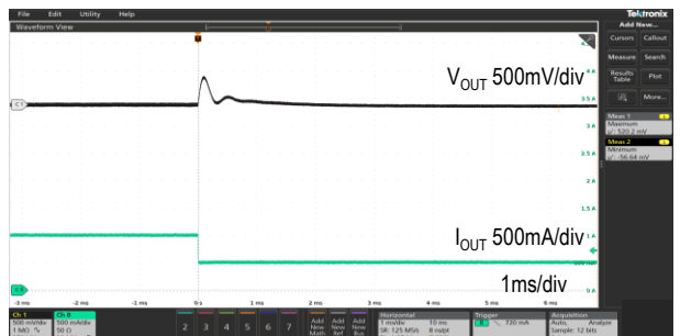
Transient Response ( V_{IN} = 48V, C_{OUT} = 22\mu F \times 4\text{pcs}, I_{OUT} = 1 \text{ to } 0.5, 0.9A/\mu s )
