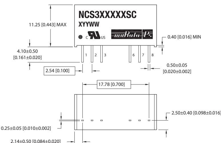
All dimensions in millimetres (inches), controlling dimension is mm.
