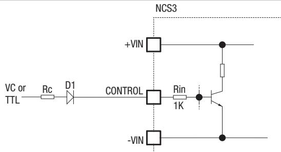
D1 (e.g. 1N4001) is necessary for correct operation of the NCS3 when the control signal is LOW. The recommended drive current  $I_b$  to shut down the NCS3 is 2 mA to 8 mA. The value of  $R_c$  can be derived as follows:
