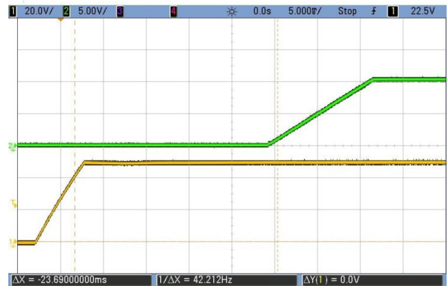
Turn-on transient at full load current (5ms/div, Top Trace: V out , 5V/div; Bottom Trace: V in , 20V/div)
