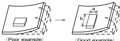
(2) Components location on PCB separation
