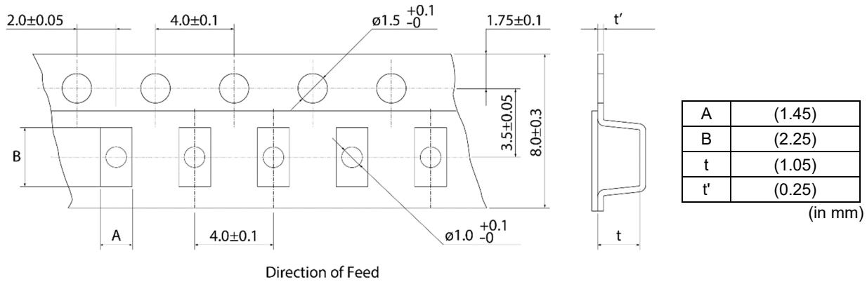
\* The dimensions of the cavity are measured at its bottom.
