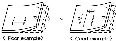
(2) Components location on PCB separation
