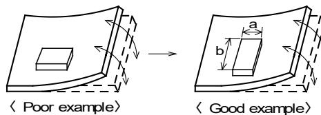
(2) Components location on PCB separation
