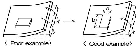
(2) Components location on PCB separation
