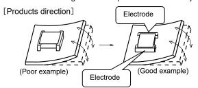
Products shall be located in the sideways direction (Length:a<b) to the mechanical stress.
