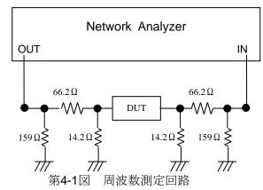
Figure 4-1 Frequency measuring circuit
