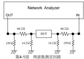
Figure 4-1 Frequency measuring circuit
