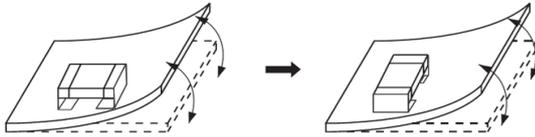
Locate chip horizontal to the direction in which stress acts.
