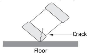
3. When printed circuit boards are piled up or handled, the corner of another printed circuit board should not be allowed to hit the capacitor, in order to avoid a crack or other damage to the capacitor.
