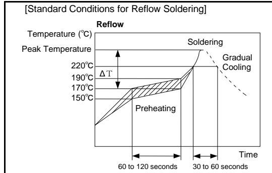
[Allowable Reflow Soldering Temperature and Time]
